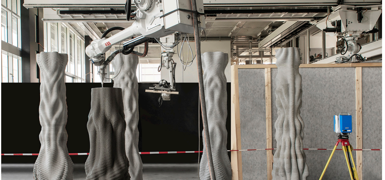
MAS ETH DFAB 20219 - Trimester 2 project - Concrete Choreography printing in the RFL
